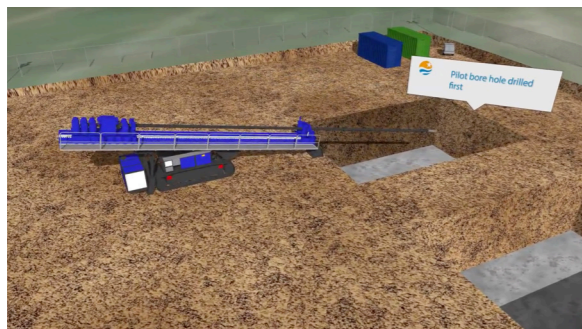
2. Excavation of joint pit, introduction of HDD rig and begin pilot bore
